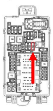
4. Remove Fuse 26, place in 2<sup>nd</sup> slot. Supplied fuse in 1<sup>st</sup>
